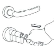
7) Securemme cylinders are equipped with projecting cam lever to offer a better hold in the event of breakage. It is possible to insert and remove the cylinder from the lock without destructive operations, only having available the keys or by turning the knob.
